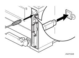
Attach the other end of the interface cable to the USB interface connector of the computer or the USB Hub. Secure the cable.
