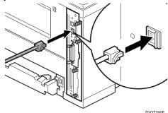
Connect the other end of the network interface cable to the network.
