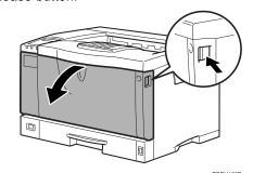
Remove the fixing material inserted between toner cartridge and the printer
