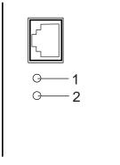
1 is lit when the printer is securely connected to the network.
