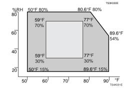
Possible operation range Recommended range The machine must be level within 5 mm, 0.2" both front to rear and left to right.
