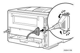
Attach the other end of the interface cable to the interface connector of the computer. Secure the cable.
